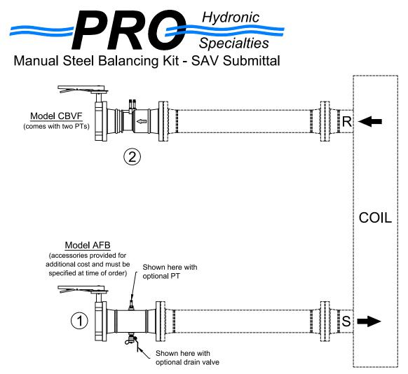
**PRODUCT DESCRIPTION:** The Manual Balancing Valve Kit is a packaged and partially preassembled grouping of components required to complete installation of a terminal unit. Temperature control valves, piping, and coils are supplied "by others". Mounting and testing of the customer provided TCV is available at an additional charge. Parts for reductions in line size are available for an additional charge. Consult with factory for information and pricing.
