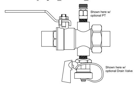
PRODUCT DESCRIPTION: The IBU is an integral ball valve and union. The IBU uses a full-port ball valve with a union ended brass body that provides two (2) 1/4" taps for accessories to be installed. All taps are plugged unless otherwise specified. Memory stops are available upon request. Fixed end connections may be SWT or FNPT. Union side connections available include MNPT, FNPT, and SWT, and a variety of reductions.
