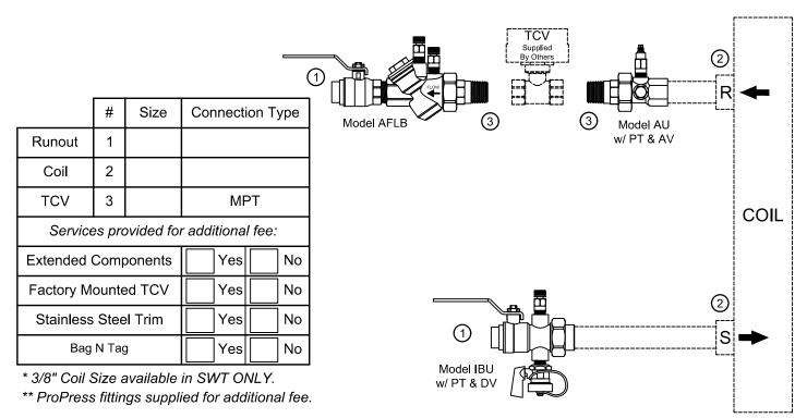
**PRODUCT DESCRIPTION:** The Automatic Balancing Valve Kit is a packaged and partially preassembled grouping of components required to complete installation of a terminal unit. Temperature control valves, piping, and coils are supplied "by others". Mounting and testing of the customer supplied TCV is available at an additional charge.
