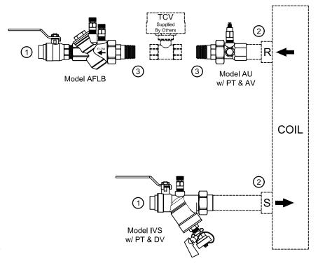
**PRODUCT DESCRIPTION:** The Automatic Balancing 2-way Valve Kit is a packaged and partially preassembled grouping of components required to complete installation of a terminal unit. Temperature control valves, piping, and coils are supplied "by others". Mounting and testing of the customer supplied TCV is available at an additional charge.
