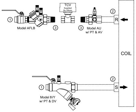
**PRODUCT DESCRIPTION:** The Automatic Balancing Valve Kit is a packaged and partially preassembled grouping of components required to complete installation of a terminal unit. Temperature control valves, piping, and coils are supplied "by others". Mounting and testing of the customer supplied TCV is available at an additional charge.
