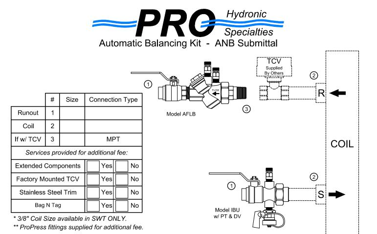
**PRODUCT DESCRIPTION:** The Automatic Balancing Valve Kit is a packaged and partially preassembled grouping of components required to complete installation of a terminal unit. Temperature control valves, piping, and coils are supplied "by others". Mounting and testing of the customer supplied TCV is available at an additional charge.
