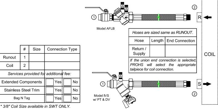
PRODUCT DESCRIPTION: The Automatic Heat Pump Hose Kit is a packaged and partially preassembled grouping of components required to complete installation of a terminal unit. Piping, and coils are supplied "by others".
