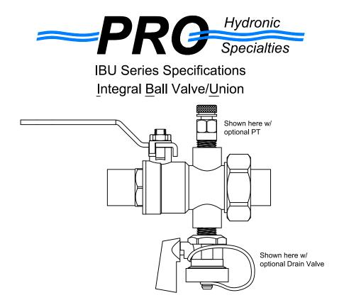
PRODUCT DESCRIPTION: The IBU is an integral ball valve and union. The IBU uses a full-port ball valve with a union ended brass body that provides two (2) ¼" taps for accessories to be installed. All taps are plugged unless otherwise specified. Memory stops are available upon request. Fixed end connections may be SWT or FNPT. Union side connections available include MNPT, FNPT, and SWT, and a variety of reductions.
