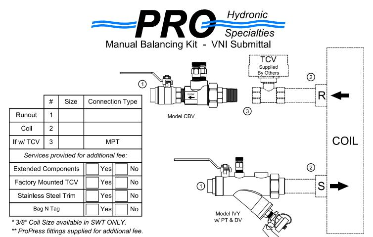
**PRODUCT DESCRIPTION:** The Manual Balancing Valve Kit is a packaged and partially preassembled grouping of components required to complete installation of a terminal unit. Temperature control valves, piping, and coils are supplied
