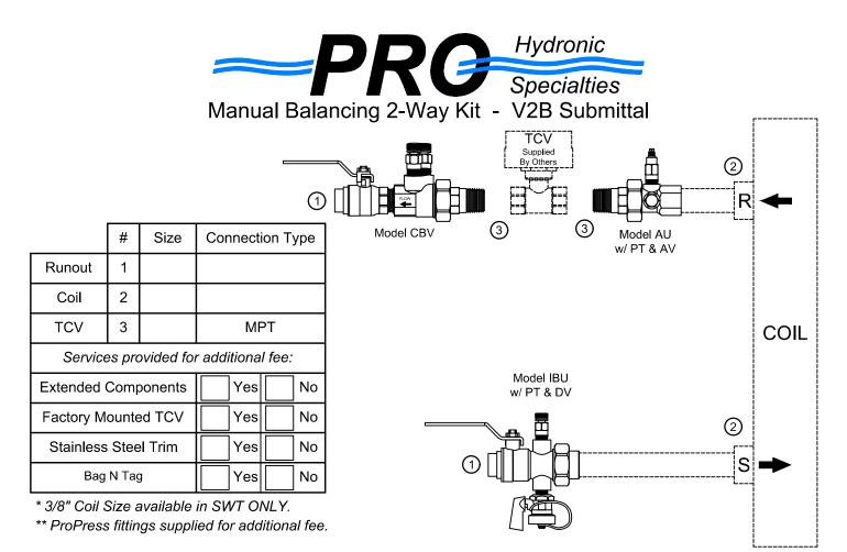
**PRODUCT DESCRIPTION:** The Manual Balancing Valve Kit is a packaged and partially preassembled grouping of components required to complete installation of a terminal unit. Temperature control valves, piping, and coils are supplied "by others". Mounting and testing of the customer supplied TCV is available at an additional charge.
