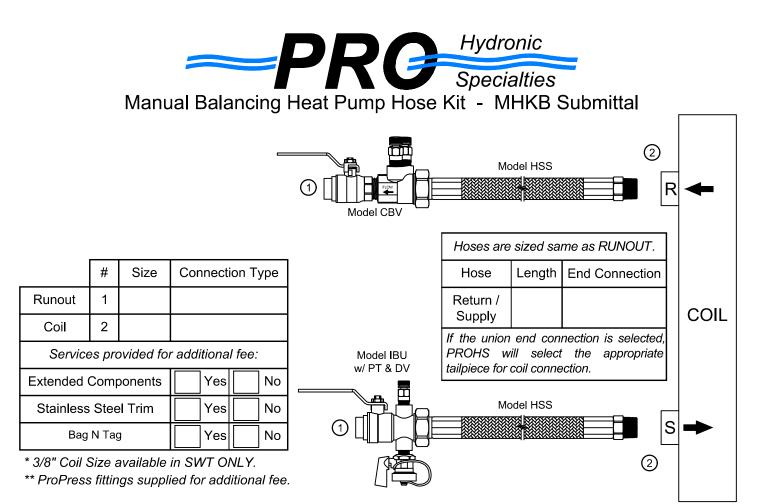
**PRODUCT DESCRIPTION:** The Manual Balancing Hose Kit is a packaged and partially preassembled grouping of components required to complete installation of a terminal unit. Temperature control valves, piping, and coils are supplied "by others". Mounting and testing of the customer supplied TCV is available at an additional charge.
