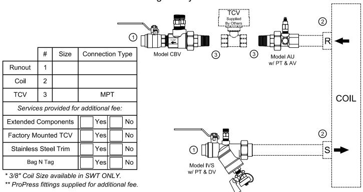
**PRODUCT DESCRIPTION:** The Manual Balancing Valve Kit is a packaged and partially preassembled grouping of components required to complete installation of a terminal unit. Temperature control valves, piping, and coils are supplied "by others". Mounting and testing of the customer supplied TCV is available at an additional charge.
