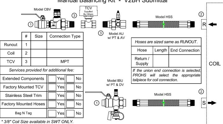
PRODUCT DESCRIPTION: The Manual Balancing Valve Kit is a packaged and partially preassembled grouping of components required to complete installation of a terminal unit. Temperature control valves, piping, and coils are supplied "by others" Mounting and testing of the customer supplied TCV is available at an additional charge
