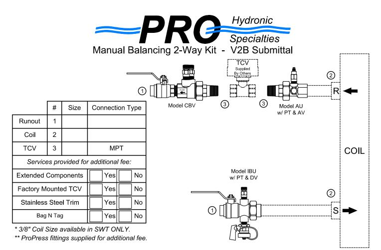
**PRODUCT DESCRIPTION:** The Manual Balancing Valve Kit is a packaged and partially preassembled grouping of components required to complete installation of a terminal unit. Temperature control valves, piping, and coils are supplied "by others". Mounting and testing of the customer supplied TCV is available at an additional charge.
