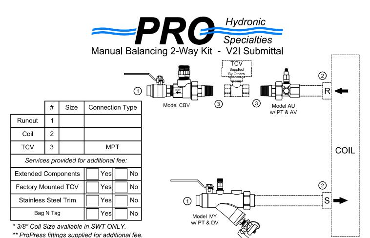
PRODUCT DESCRIPTION: The Manual Balancing Valve Kit is a packaged and partially preassembled grouping of
