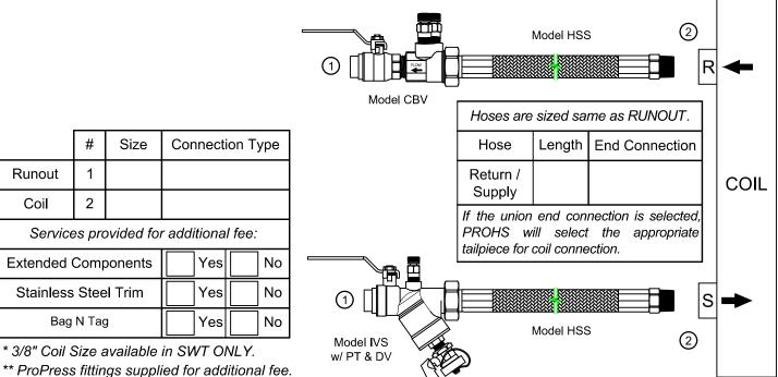
**PRODUCT DESCRIPTION:** The Manual Balancing Hose Kit is a packaged and partially preassembled grouping of components required to complete installation of a terminal unit. Temperature control valves, piping, and coils are supplied "by others". Mounting and testing of the customer supplied TCV is available at an additional charge.
