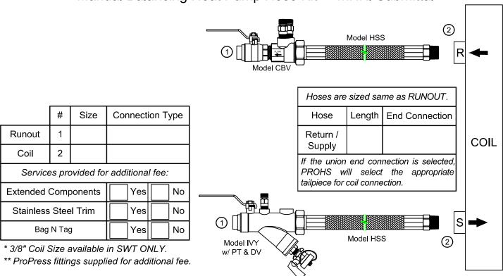
**PRODUCT DESCRIPTION:** The Manual Balancing Hose Kit is a packaged and partially preassembled grouping of components required to complete installation of a terminal unit. Temperature control valves, piping, and coils are supplied "by others". Mounting and testing of the customer supplied TCV is available at an additional charge.
