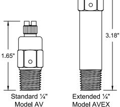
PRODUCT DESCRIPTION: The model AV is a manual air vent that is both knurled and slot operated. The model AV allows for manual purging of air from systems. The AV has a blowout proof stem.
