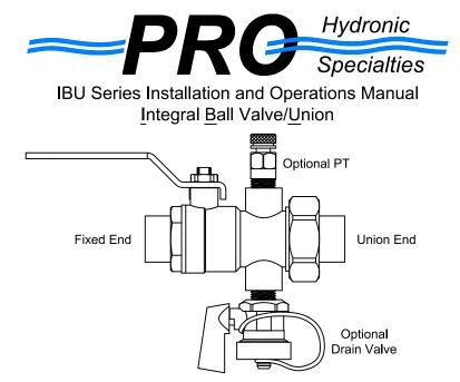
PRODUCT DESCRIPTION: The IBU is an integral ball valve/union that is rated at 600 WOG / CWP. The IBU uses a combination full-port ball valve and union which provides two (2) 1/4" taps for accessories to be installed. All taps are plugged unless otherwise specified. Fixed end connections may be SWT or NPTF. Union side connections available include NPTM, NPTF, and SWT, and a variety of reductions.
