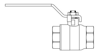
PRODUCT DESCRIPTION: The BV is a brass ball valve rated at 600 WOG / CWP. And comes with SWT or FNPT connections.
