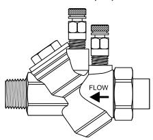
PRODUCT DESCRIPTION: The AFLD is an Automatic Pressure Independent Flow Limiting device, male ended by union, rated at 600 WOG / CWP @ 250°F. The AFLD is supplied with a stainless steel flow limiting cartridge that can be removed for cartridge exchange if necessary. The AFLD comes standard with two P/T ports and a hanging ID tag for easy identification. The union side connections available are NPTM, NPTF, SWT, and a variety of reductions.
