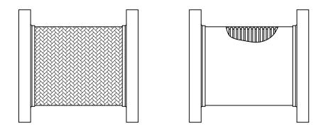
PRODUCT DESCRIPTION: The Model PCS is a flexible pump connector that offers numerous advantages when installed in piping systems. The PCS contains a flexible stainless steel corrugated inner hose that is covered with a stainless steel braid. The PCS helps to extend the life of a pump in a piping system by providing vibration isolation and stress relief from misalignment, and it also reduces noise from operation. The PCS comes with ANSI 150# Class flanges.
