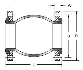
PRODUCT DESCRIPTION: The Model REJ is an EPDM Single Ball rubber expansion joint with ANSI Class 150# Flanges that offers numerous advantages when installed in piping systems. The REJ helps to reduce noise and vibration from mechanical equipment, as well as compensating for misalignment of equipment due to operation and installation. The REJ also provides relief from expansion and contraction of systems due to varying temperatures. Available in 2½", 3", 4", 6" and 8" sizes.
