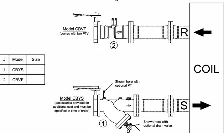
**PRODUCT DESCRIPTION:** The Manual Balancing Valve Kit is a packaged and partially preassembled grouping of components required to complete installation of a terminal unit. Temperature control valves, piping, and coils are supplied "by others". Mounting and testing of the customer provided TCV is available at an additional charge. Parts for reductions in line size are available for an additional charge. Consult with factory for information and pricing.
