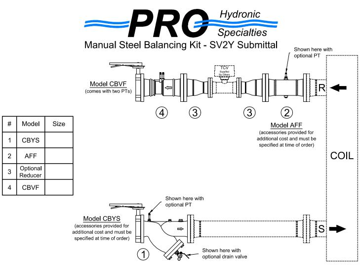
**PRODUCT DESCRIPTION:** The Manual Balancing Valve Kit is a packaged and partially preassembled grouping of components required to complete installation of a terminal unit. Temperature control valves, piping, and coils are supplied "by others". Mounting and testing of the customer provided TCV is available at an additional charge. Parts for reductions in line size are available for an additional charge. Consult with factory for information and pricing.
