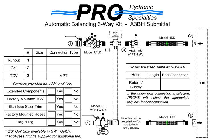
**PRODUCT DESCRIPTION:** The Automatic Balancing Valve Kit is a packaged and partially preassembled grouping of components required to complete installation of a terminal unit. Temperature control valves, piping, and coils are supplied "by others". Mounting and testing of the customer supplied TCV is available at an additional charge.
