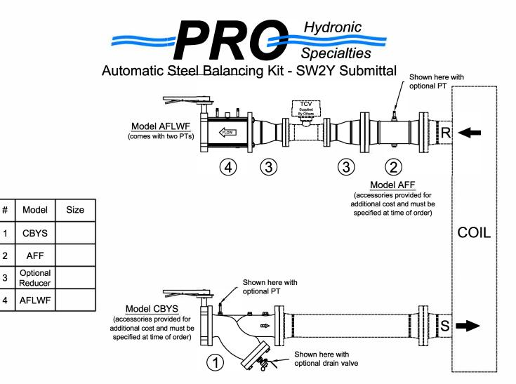
**PRODUCT DESCRIPTION:** The Automatic Balancing Valve Kit is a packaged and partially preassembled grouping of components required to complete installation of a terminal unit. Temperature control valves, piping, and coils are supplied "by others". Mounting and testing of the customer provided TCV is available at an additional charge. Parts for reductions in line size are available for an additional charge. Consult with factory for information and pricing.
