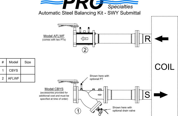
PRODUCT DESCRIPTION: The Automatic Balancing Valve Kit is a packaged and partially preassembled grouping of components required to complete installation of a terminal unit. Temperature control valves, piping, and coils are supplied "by others". Mounting and testing of the customer provided TCV is available at an additional charge. Parts for reductions in line size are available for an additional charge. Consult with factory for information and pricing.
