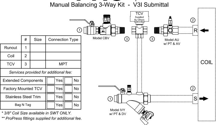
**PRODUCT DESCRIPTION:** The Manual Balancing Valve Kit is a packaged and partially preassembled grouping of components required to complete installation of a terminal unit. Temperature control valves, piping, and coils are supplied "by others". Mounting and testing of the customer supplied TCV is available at an additional charge.
