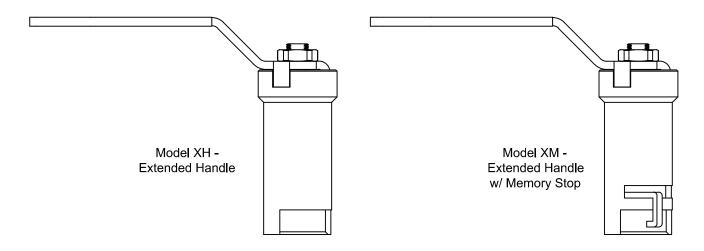
PRODUCT DESCRIPTION: The extended handle is designed to ensure stable operation of a valve while elevating the handle in order to allow for piping insulation. The extended handle can accommodate  $\frac{1}{2}$ " through  $\frac{2}{2}$ " valve sizes. The extended handle is available with a groove for a memory stop (Model XM) or without (Model XH).
