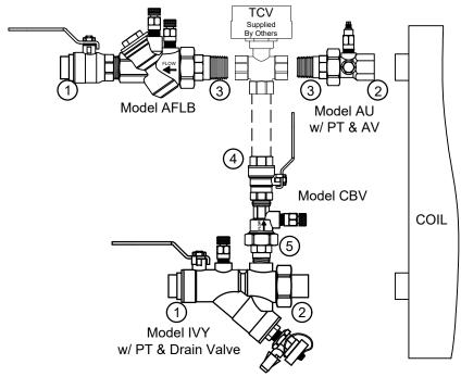
**PRODUCT DESCRIPTION:** The A3IV Automatic Balancing 3-way Valve Kit is a packaged and partially preassembled grouping of components required to complete installation of a terminal unit. Temperature control valves, piping, and coils are supplied "by others". Mounting and testing of the customer supplied TCV is available at an additional charge.
