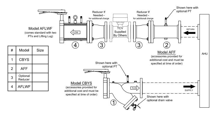
**PRODUCT DESCRIPTION:** The SW2Y Automatic Balancing Valve Kit is a packaged and partially preassembled grouping of components required to complete installation of a terminal unit. Temperature control valves, piping, and coils are supplied "by others". Mounting and testing of the customer provided TCV is available at an additional charge. Parts for reductions in line size are available for an additional charge. Consult with factory for information and pricing.
