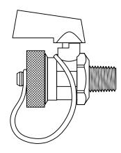
PRODUCT DESCRIPTION: The Model DV is a hose-end drain valve that is designed for quick and easy draining of a piping system or component. The drain valve incorporates a mini-ball for on and off functioning, and has removable cap where a  $\frac{3}{4}$ " GHT hose can be connected. The drain valves are available in  $\frac{1}{4}$ " MNPT,  $\frac{1}{2}$ " MNPT, and  $\frac{3}{4}$ " MNPT end connections.
