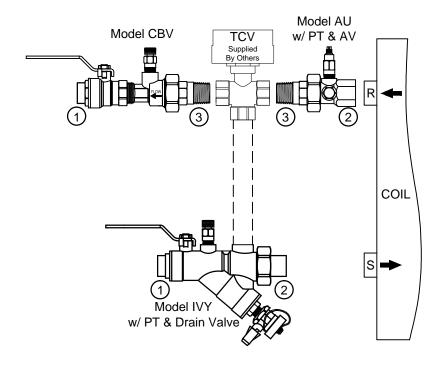
**PRODUCT DESCRIPTION:** The V3I Manual Balancing 3-way Valve Kit is a packaged and partially preassembled grouping of components required to complete installation of a terminal unit. Temperature control valves, piping, and coils are supplied "by others". Mounting and testing of the customer provided TCV is available at an additional charge. No bypass device is included with the V3I kit but may be supplied at an additional charge.
