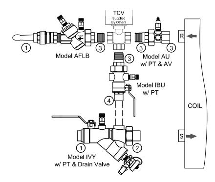
PRODUCT DESCRIPTION: The A3IB Automatic Balancing 3-way Valve Kit is a packaged and partially preassembled grouping of components required to complete installation of a terminal unit. Temperature control valves, piping, and coils are supplied "by others". Mounting and testing of the customer supplied TCV is available at an additional charge.
