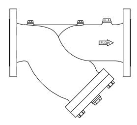
PRODUCT DESCRIPTION: The CYS is a flange x flange end wye strainer with Class 150# flange ends. The wye strainer comes standard with a stainless steel perforated filter element, (2)  $\frac{1}{4}$ " plugs, (1)  $\frac{1}{2}$ " plug, (1) plugged  $\frac{3}{4}$ " blow-off connection, and a flanged blow-off cover with an EPDM o-ring. Accessories (pressure/temperature ports, manual air vents, and drain valves) are available for an additional cost.
