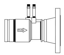
PRODUCT DESCRIPTION: The SGVF is a grooved by flange style venturi. The grooved end carbon steel venturi connects to a standard ANSI Class 150 pound flange. The venturi is designed for highly accurate flow measurement with low pressure loss. High and low flow ranges are available in the  $2\frac{1}{2}$ ", 3", and 4" sizes. The SGVF comes standard with two pressure/temperature ports.
