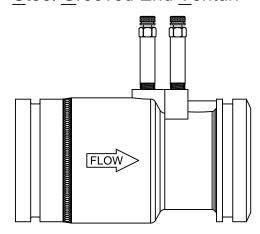
PRODUCT DESCRIPTION: The SGV is a steel Venturi with grooved ends that is designed for highly accurate flow measurement with low pressure loss. High and low flow ranges are available in the 2½", 3", and 4" sizes. The SGV comes standard with two pressure/temperature ports.
