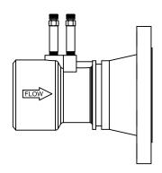
PRODUCT DESCRIPTION: The SWVF is a weld end by flange end style steel venturi. The carbon steel venturi connects to a standard ANSI Class 150 pound flange. The venturi is designed for highly accurate flow measurement with low pressure loss. High and low flow ranges are available in the  $2\frac{1}{2}$ ", 3", and 4" sizes. The SWVF comes standard with two pressure/temperature ports.
