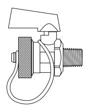
PRODUCT DESCRIPTION: The Model DV is a hose-end drain valve that is designed for quick and easy draining of a piping system or component. The drain valve incorporates a mini-ball for on and off functioning, and has removable cap where a <sup>3</sup>/<sub>4</sub>" GHT hose can be connected. The drain valves are available in <sup>1</sup>/<sub>4</sub>" MNPT, <sup>1</sup>/<sub>2</sub>" MNPT, and <sup>3</sup>/<sub>4</sub>" MNPT end connections.
